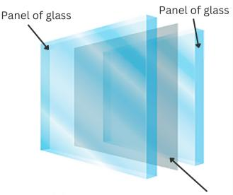
Sheet of flexible interlayer sandwiched and bonded between two glass panels
